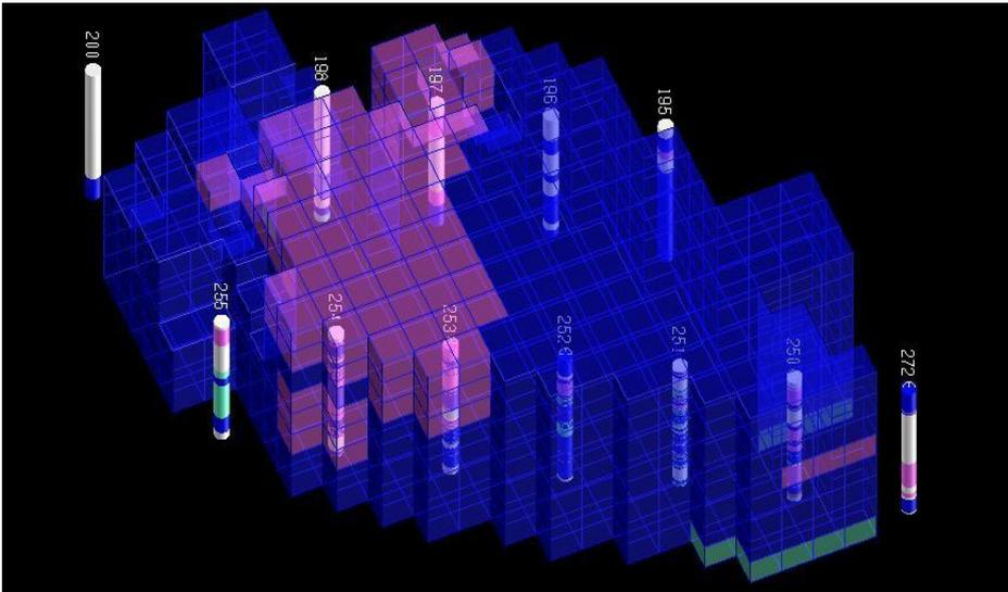
**Fig.6 BSA block model, 3X3X3 meter blocks**
