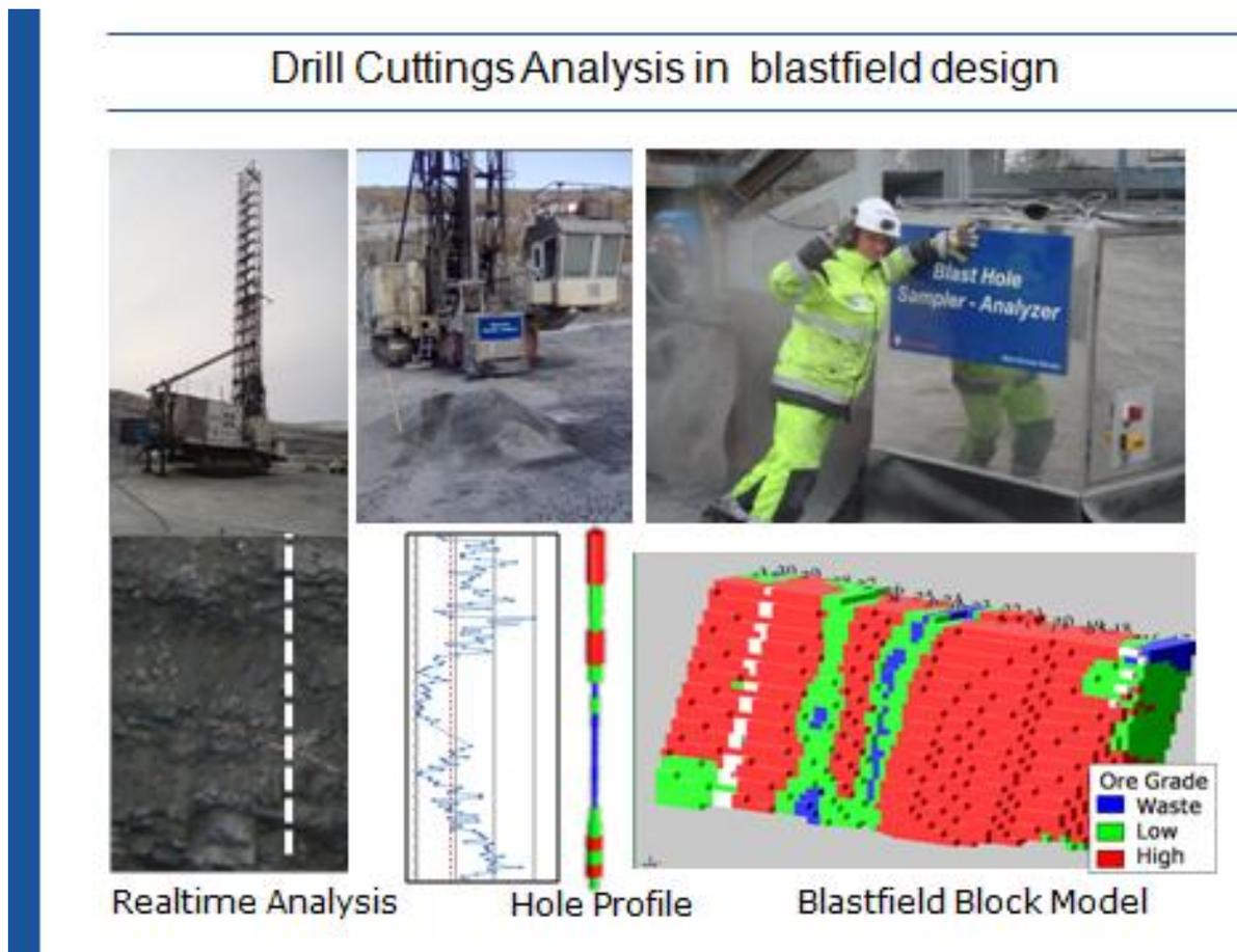
**Figure 5. Blast Hole Sampler-Analyzer (BSA) in blast field design**
