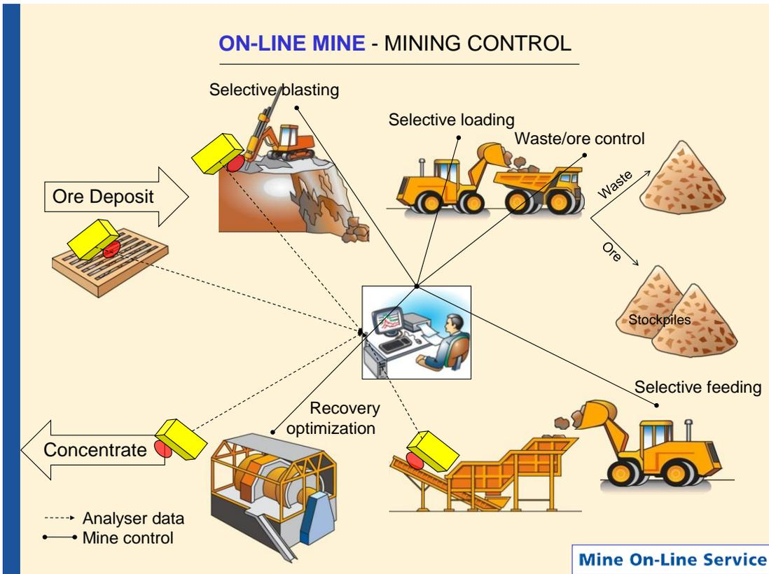
**Fig. 8. On-Line Mine information network**
