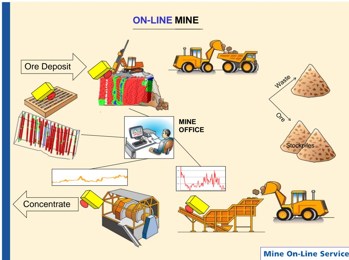
Fig. 2. The On-Line Mine analysis points (yellow boxes)
