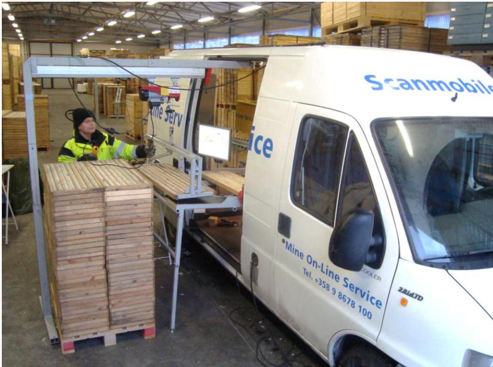
**Fig. 3 The Scanmobile operating in drill core storage**
