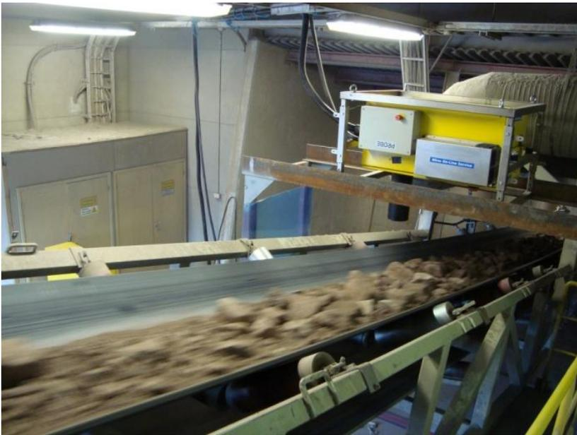
**Fig. 7. LIF Cross Belt analyser**
