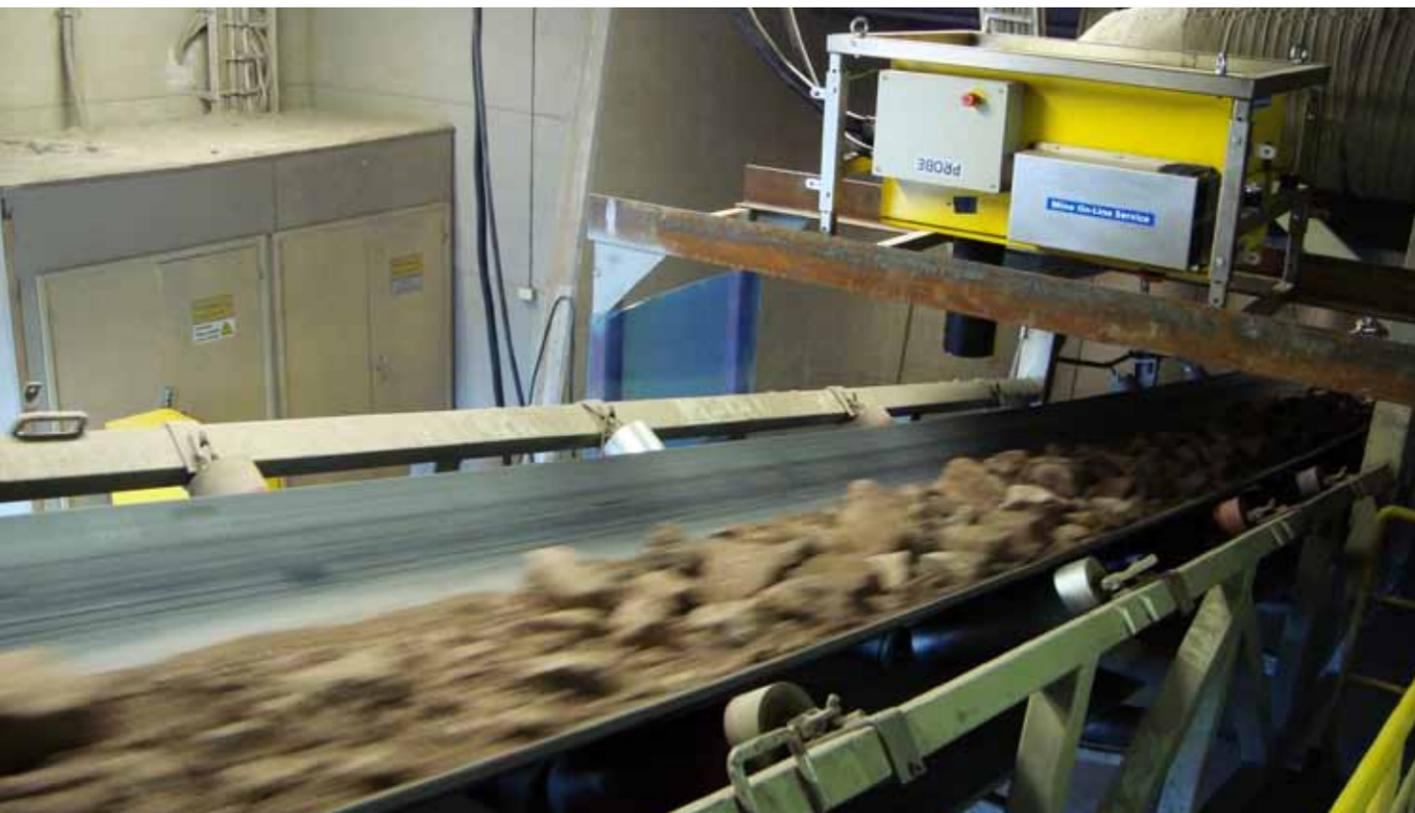
OreSpex on conveyor detecting waste
